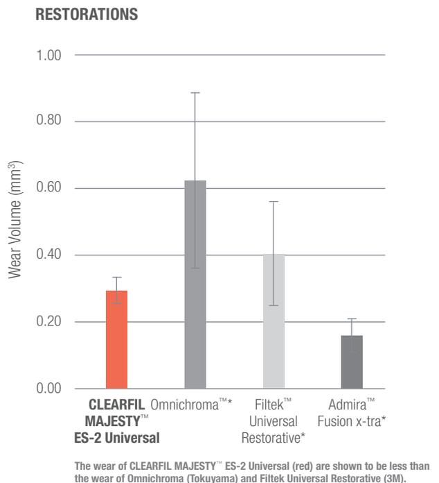
Test Conditions: Leinfelder wear test at room temperature in water. Load: 7.9 kg/cm², 400,000 cycles. Antagonist: bovine enamel, polished with #3000 paper. Material: polished with #3000 paper.
